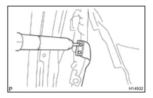
(b) Rivet the band on the link using a pneumatic riveter or hand riveter.
