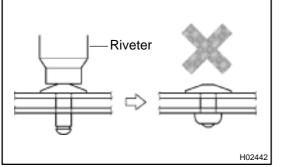
Do not tilt the riveter and disconnect the rivet from the material while operating a riveter otherwise, the materials could not be tightened firmly.
